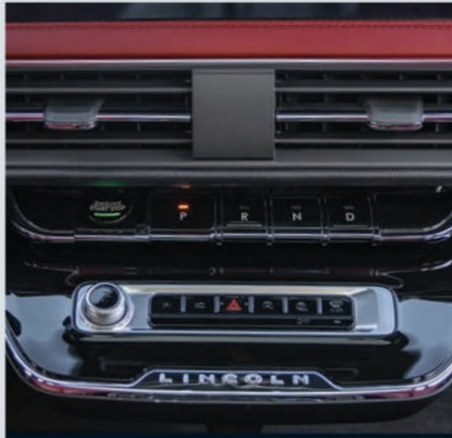
2023 LINCOLN CORSAIR The Lincoln's shifter is almost impossible to operate without looking.
